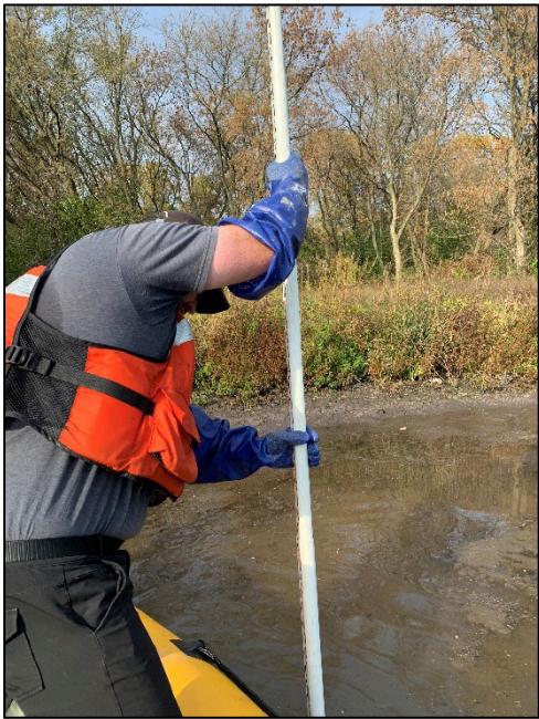
Figure 5 Liner measurements taken using a GNSS-mounted survey rod.
