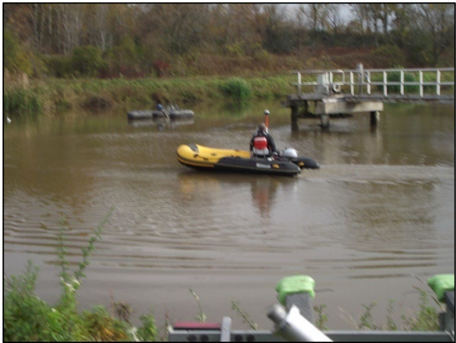
Figure 3 Sludge Mapper vessel and sonar system on the lagoon.
