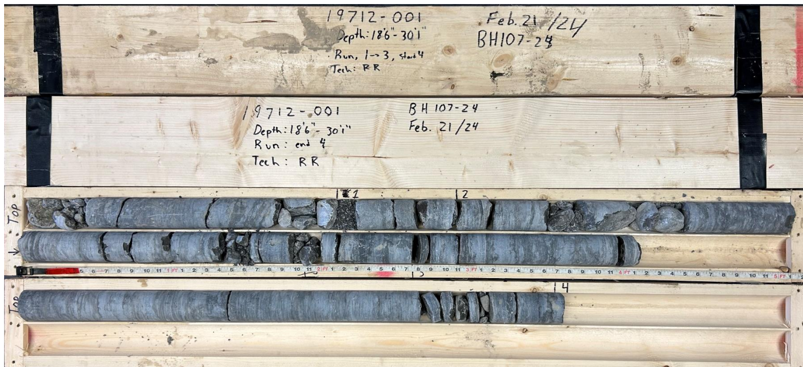
Photo 3: Rock Core Run 1-4, BH107-24, 5.0 to 9.2 mbgs
