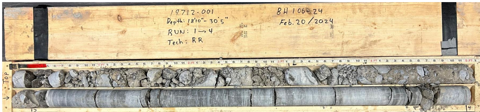
Photo 2: Rock Core Run 1-4, BH106-24, 5.7 to 9.3 mbgs
