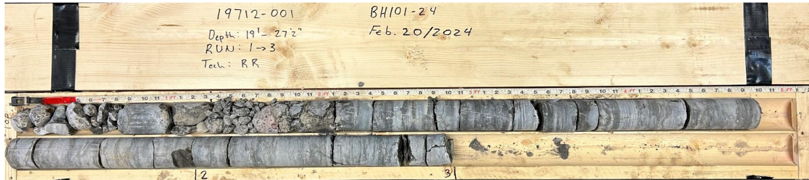
Photo 1: Rock Core Run 1- 3, BH101-24, 5.8 to 8.3 mbgs
